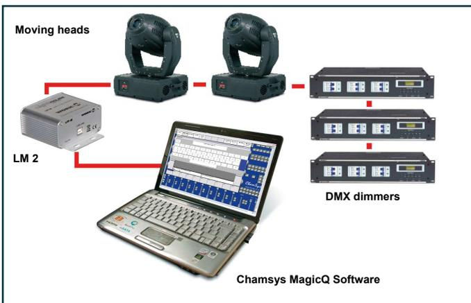
Connection system using **LM 2** as lighting controller. From a computer and MagicQ ChamSys software is possible to create any type of installation to lighting system control, as much spots as robots.
