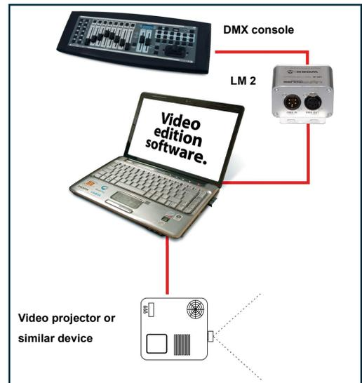
**LM 2** connecting to operate as Media Server from a physical console, it is possible to run video, edit and mix with a video editing software.
