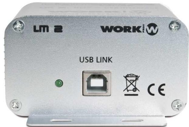
**LM 2** is a bi-directional DMX / USB interface that allowing, the manage the signal in both directions, to operate as two different devices:
